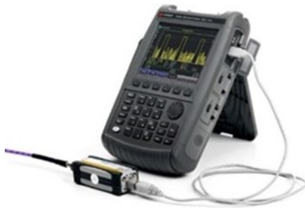
Simplify power measurements with USB power sensors
