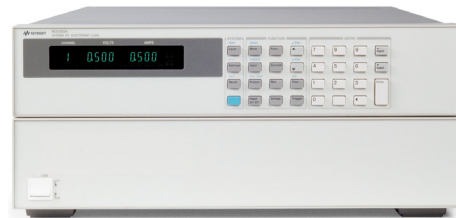
DC electronic load mainframe
