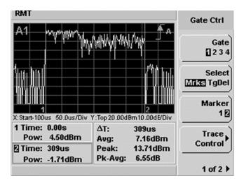
Figure 8. WiMAX burst signal capture
