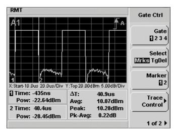
Figure 5. Markers 1 and 2 time and power, with  $\Delta$  time and power measurements between markers.
