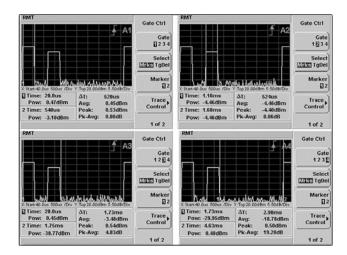
Figure 7. Measurement flexibility with 4 independent time gates
