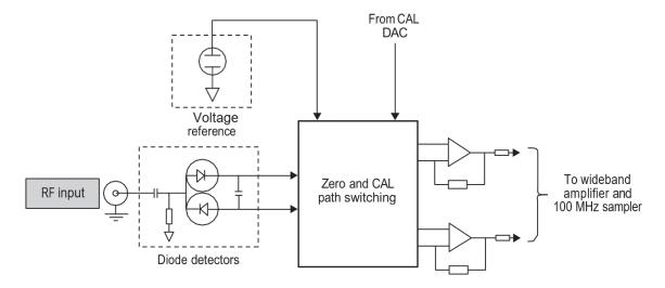
Figure 1. Internal zero and cal block diagram
